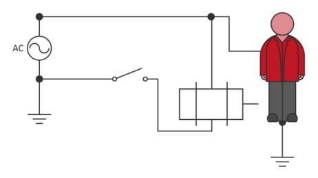
If properly wired to switch the "Hot" conductor there are circumstances where the neutral can be charged
