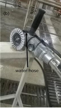
Figure 2 – (a) A handheld pneumatic wet polisher used in the polishing process; (b) A handheld pneumatic wet grinder with a diamond grinding cup wheel in the final grinding process.
