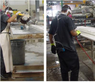
Figure 1 – (a) A worker using a handheld pneumatic wet grinder with a diamond grinding cup wheel in the final grinding process; (b) A worker using a handheld pneumatic wet polisher in the polishing process; (c) A worker using a wet miter saw in the lamination process; (d) A worker using compressed air to dry the surface of the stone in the lamination process.
