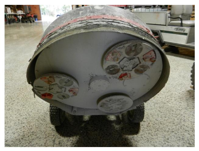
Figure 4: Shroud and polishing disks installed on the Concrete Polisher
