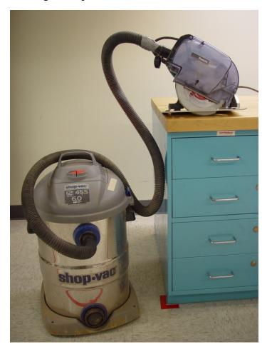
Figure 4 –The dust-collecting circular saw and its connection to the shop vacuum used in this survey. Photo courtesy of NIOSH.
