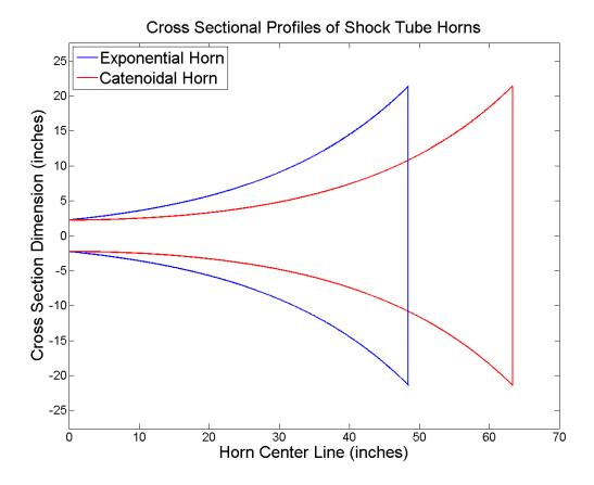
Figure 19: Catenoidal and exponential center-line cross-section profile of the horn
