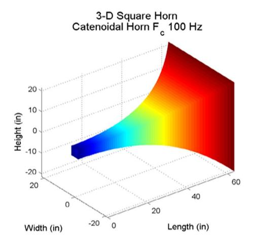
Figure 22: Three-dimensional rendering of the catenoidal horn
