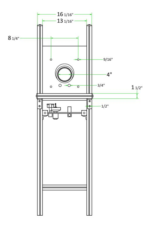
Figure 4: Front view of acoustic shock tube
