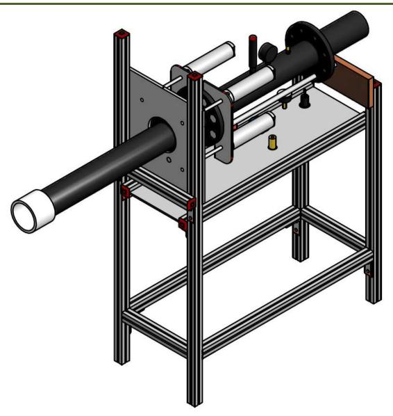
Figure 2: Three-dimensional mechanical rendering of the acoustic shock tube
