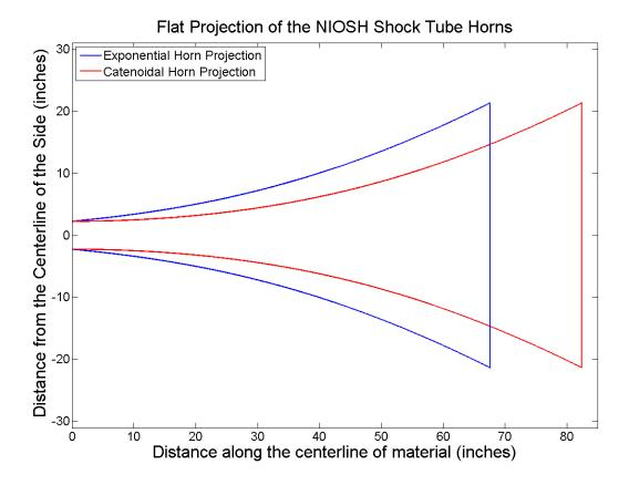
Figure 20: Catenoidal and exponential sides of the horn projected onto a flat surface
