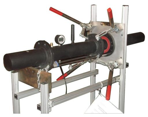
Figure 1: Second prototype acoustic shock tube
