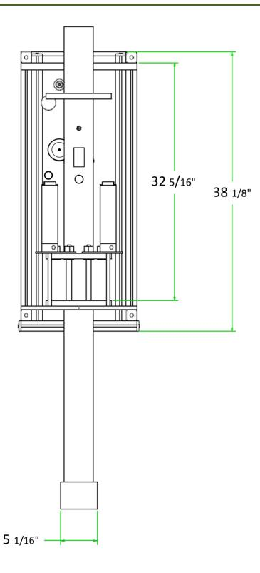
Figure 5: Top view of acoustic shock tube
