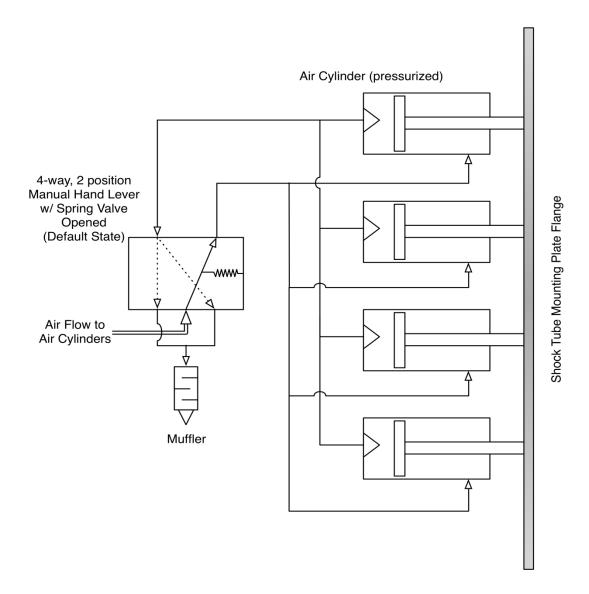
Figure 16: Pressurized shock tube with clamped membrane airflow diagram
