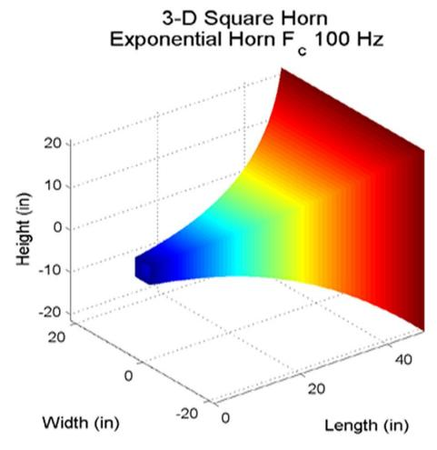
Figure 21: Three-dimensional rendering of the exponential horn
