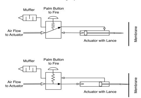
Figure 18: Pneumatic lance system for puncturing the membrane
