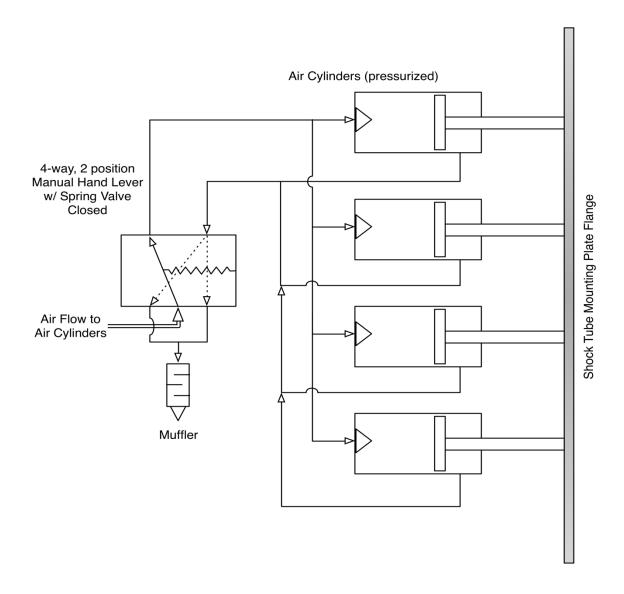
Figure 15: Unpressurized shock tube with unclamped membrane airflow diagram
