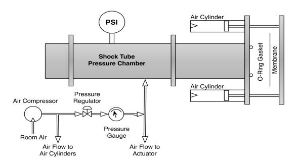
Figure 17: Shock tube pressurization system
