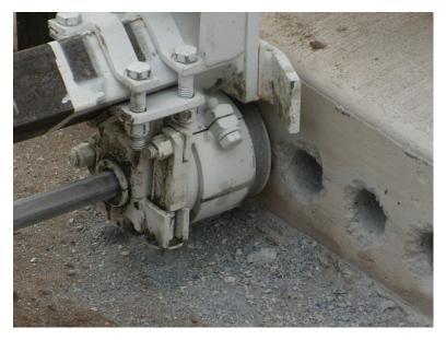
Figure 3 – Hood Surrounding Drill Steel at Concrete Surface
