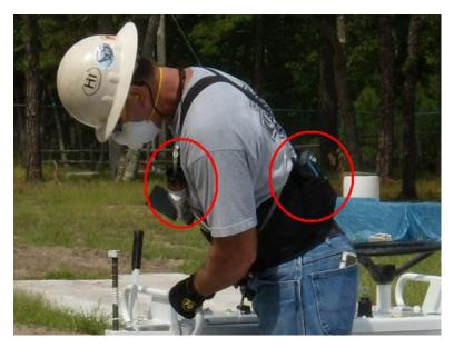
Figure 2 – Laborer Wearing Pump and Cyclone (Circled)
