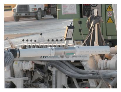
Figure 5 - Air Flow Measurement Device on Company-Owned Drill
