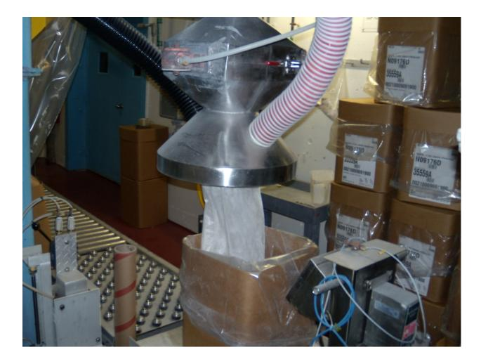
Figure 6. Engineering control outfitted on the packaging lines
