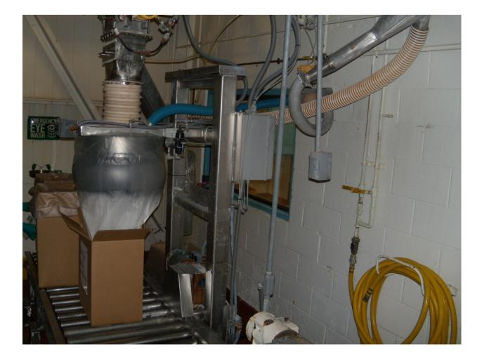
Figure 7. Inflatable seal for the packaging lines
