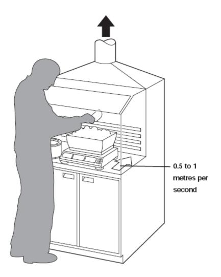
Figure 9. Ventilated Bag Dumping/Emptying Station, 1.0 mps is equivalent to 200 fpm. Contains public sector information published by the Health and Safety Executive and licensed under the Open Government License v1.0.
