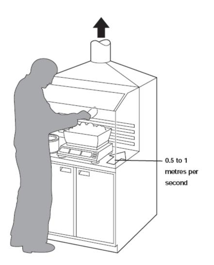
Figure 5. Bench-top ventilation for weighing/handling powders (HSE FL02) (0.5-1 m/s is equivalent to 100-200 fpm). Contains public sector information published by the Health and Safety Executive and licensed under the Open Government Licence v1.0.
