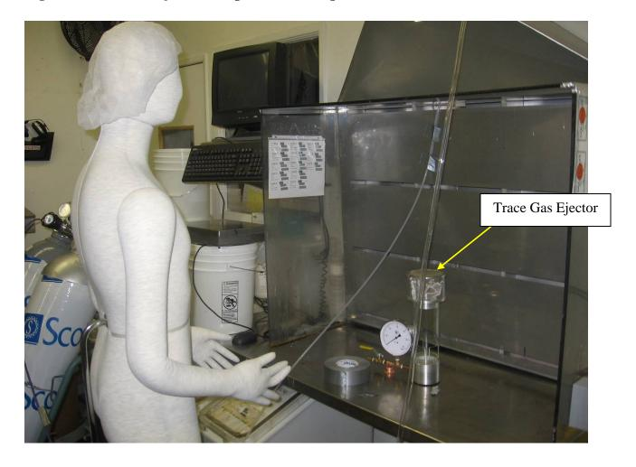
Figure 6. SF6 source coil for booth testing.
