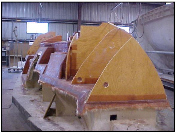
Figure 4: Internal Glass Unit (IGU)
