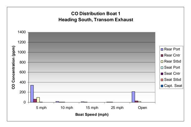
Figure 2: CO Distribution from Indmar Technology heading South
