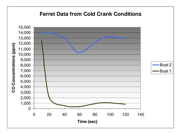
**Figure 8: Ferret Data Measured Directly Into the Exhaust Opening**
