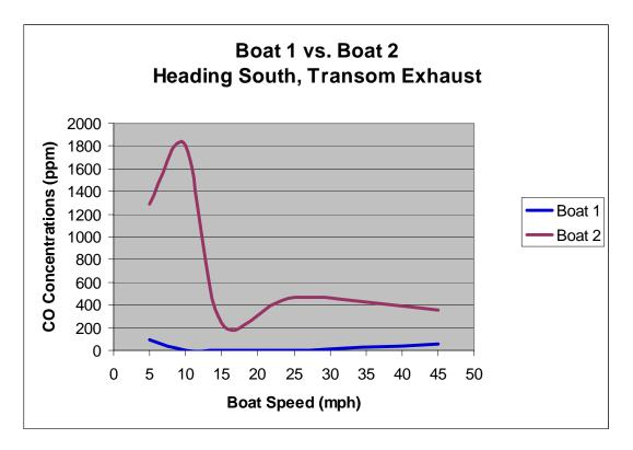
Figure 6: Comparison of CO Distribution from PAC III Data heading South
