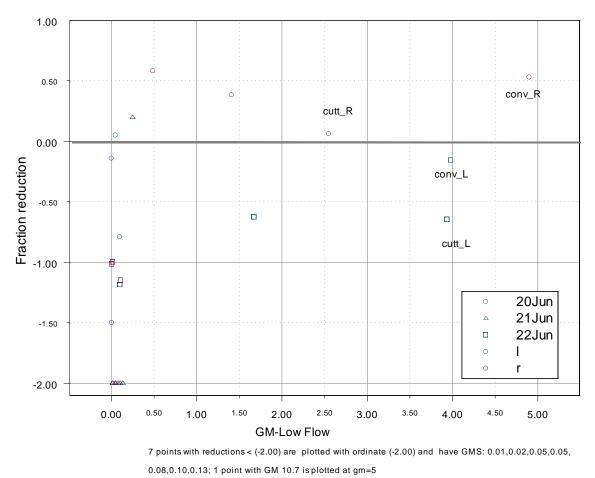
Circle, June 20, 2006; triangle, June 21, 2006; square, June 22, 2006. Blue, left side; red, right side.  $conv_R = conveyor right; conv_L = conveyor left; cutt_R = cutter right; cutt_L = cutter left$ Note: *Negative reduction values indicate* increases *in concentration*.
