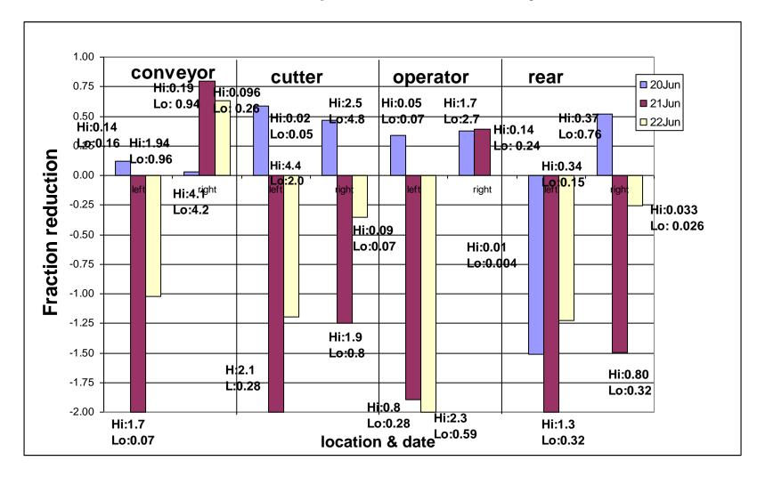
Notes: (1) Negative reduction values indicate increases in concentration. (2) Data for operator-right location on June 22 missing due to equipment problem.
