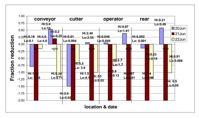
Notes: Negative values indicate *increases* in concentration. Bars cut off at -2.00 indicate values less than -2.00. Data for operator-right location on June 22 missing due to equipment problem.
