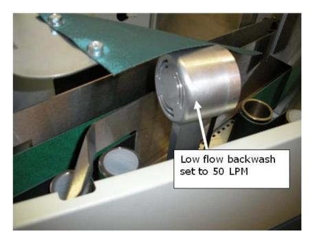
Figure 3: Low-flow backwash orifice set to 50 ALPM
