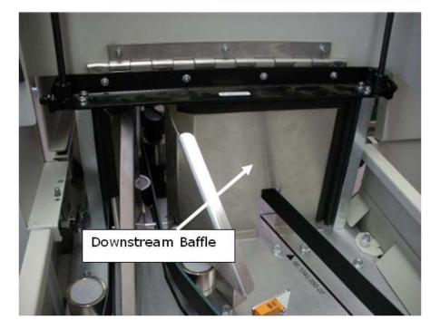
Figure 2: Downstream baffle near the second cover
