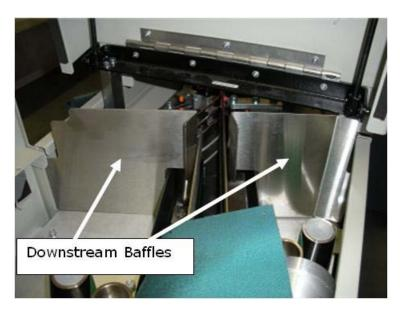
Figure 1: Downstream baffle near the first cover
