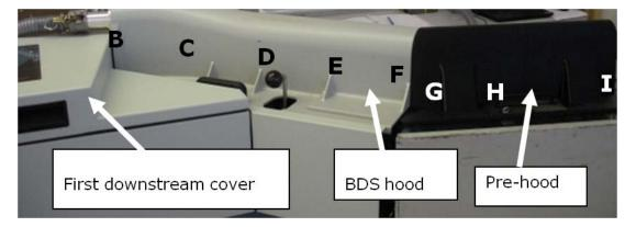
Figure 6: Tracer gas release locations B through I for the BDS hood of the AFCS 200
