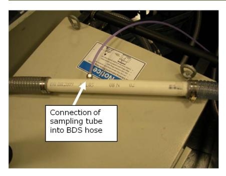
Figure 5: Connection of sampling tube to the BDS hose
