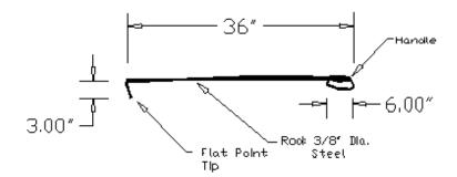
Figure 13. Sorting Parts Hook
