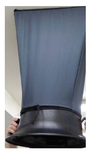
Figure 6. TSI Accubalance® Plus Air Capture Hood (Photo Credit: NIOSH)
