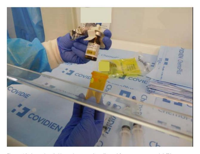
Figure 12. Intentional "Hot" wipe sample collected from mustargen vial (Photo credit: NIOSH)
