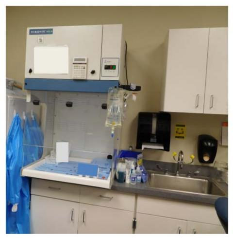
Figure 2. Ductless fume hood, Misonex Aura 30L Series Model AU-30L. Also shown: disposable gowns, sink, and toceranib bottle in white bin. (Photo Credit: NIOSH)
