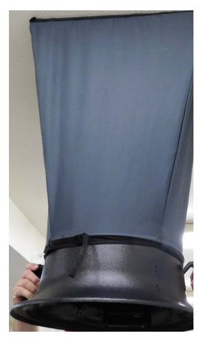
Figure 9. TSI Accubalance® Plus Air Capture Hood (Photo Credit: NIOSH)
