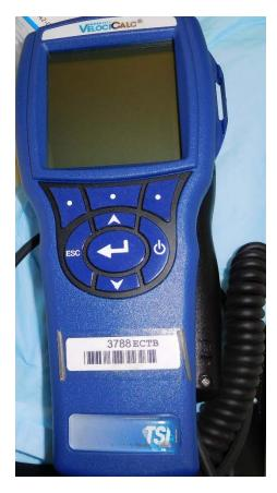
Figure 7. TSI® VelociCalc™ Plus Model 9565-P thermal anemometer (Photo Credit: NIOSH)
