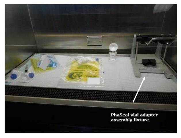
Figure 3. Class II Type A2 Model BBF-3SSRX. Also shown: PhaSeal vial adapter and disposable absorbent pad. (Photo credit: NIOSH)
