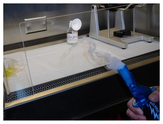
Figure 8. Qualitative smoke test with Wizard Stick Smoke Generator (Photo Credit: NIOSH)
