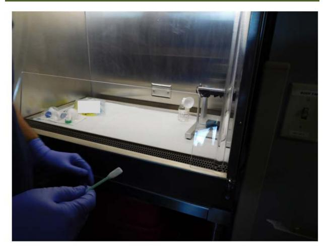
Figure 32. Wipe sample collection from random spots on BSC front surface (Photo Credit: NIOSH)
