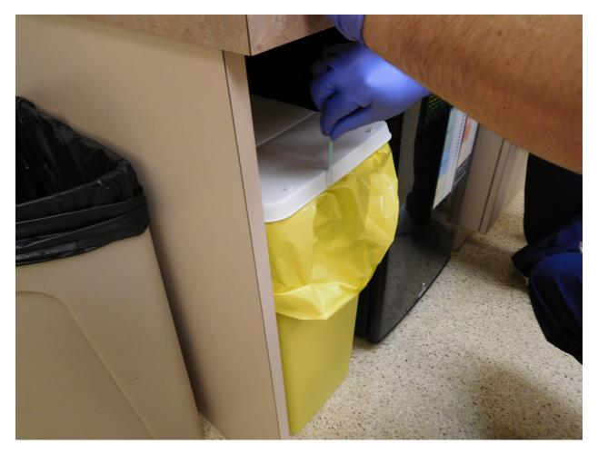
Figure 13. Surface wipe sample collected from chemotherapy waste bin (Photo Credit: NIOSH)
