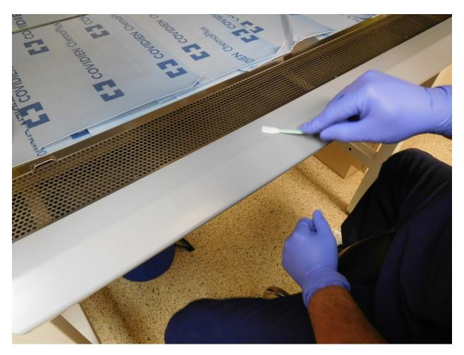
Figure 9. Surface wipe sample collected on BSC's airfoil and lip (Photo Credit: NIOSH)
