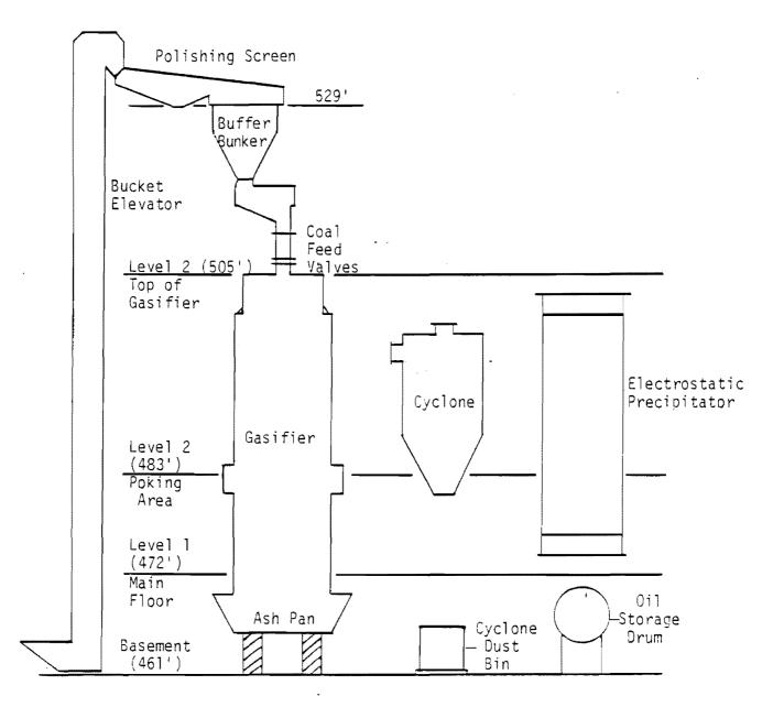
Figure 2. Major Levels in the Gasifier Building at the UMD Heating Plant.
