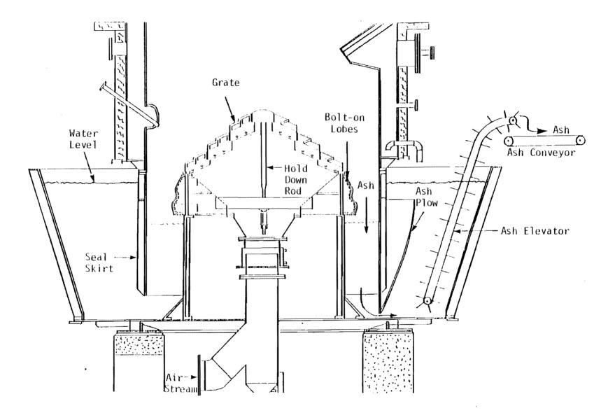
Figure 5. Diagram of the Ash Removal Mechanism
