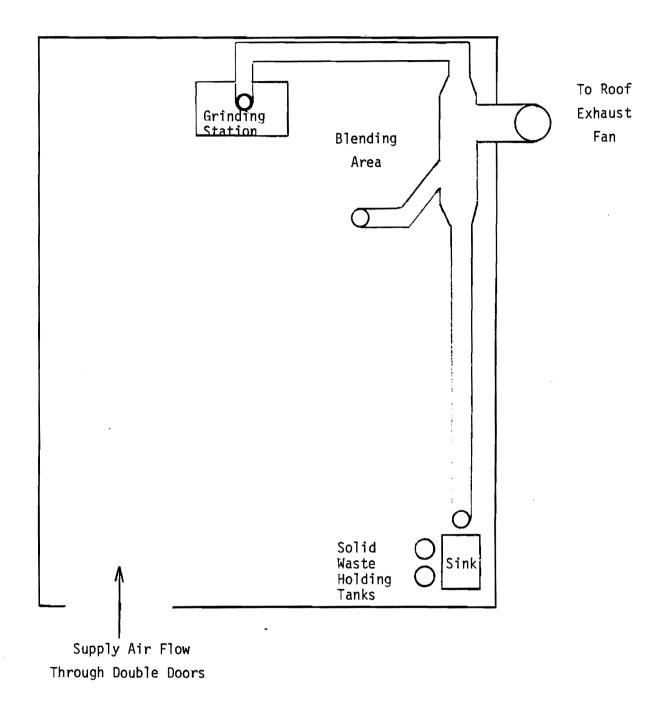
Figure 2. Gel Room Ventilation System
