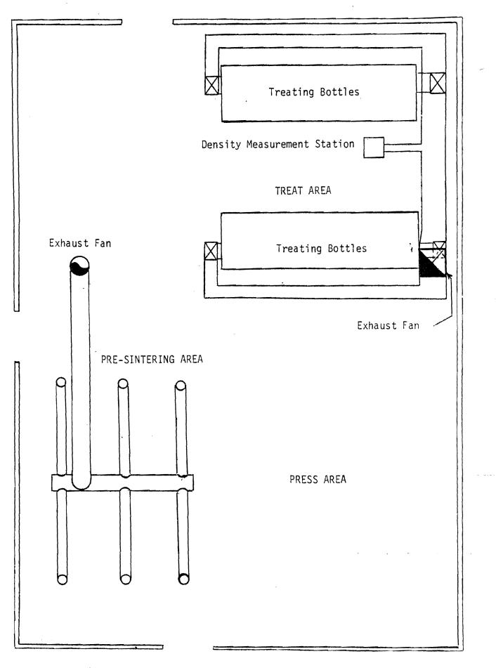
Figure 2. Press and Treat Room - Air Exhaust System.
