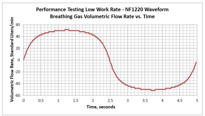
Figure 4: Example graph for Low Work Rate, showing breathing gas volumetric flow rate (y-axis) vs. time (x-axis).
