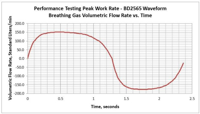
Figure 2: Example graph for Peak Work Rate, showing breathing gas volumetric flow rate (y-axis) vs. time (x-axis).
