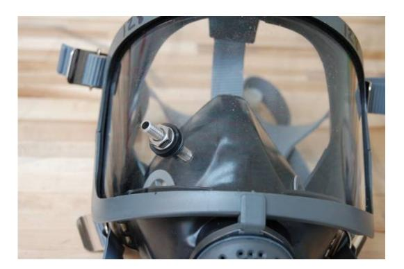
Figure 8: Exterior View of a Probed Sample Respirator
