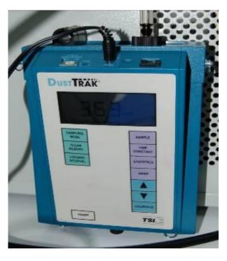
Figure 3: Dustrack Aerosol Monitor
