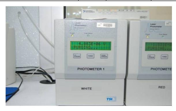
Figure 1: Laser Photometer, Model 8587A
