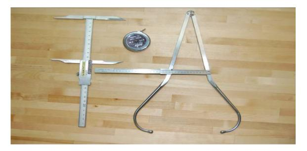
Figure 6: Facial Size Measurement Calipers
