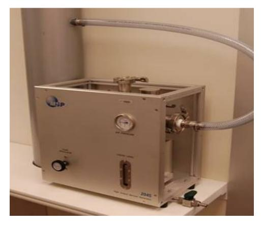
Figure 2: Aerosol Generator
