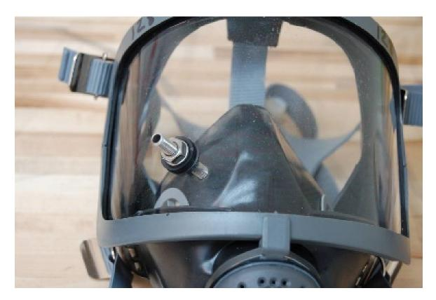
Figure 9: Exterior View of a Probed Sample Respirator
