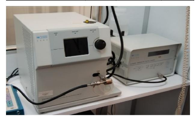
Figure 5: Scanning Mobility Particle Sizer
