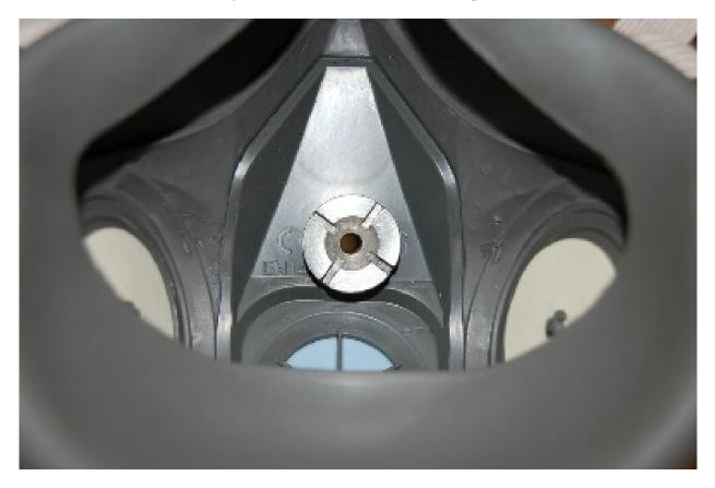
Figure 8: Interior View of a Probed Sample Respirator
