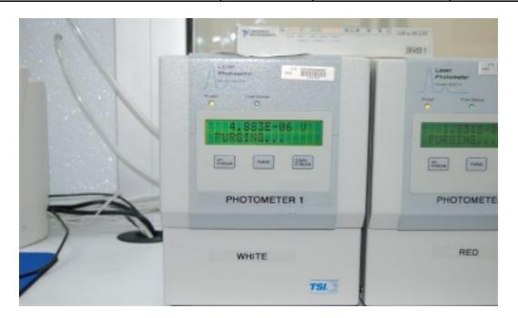
Figure 1: Laser Photometer, Model 8587A
