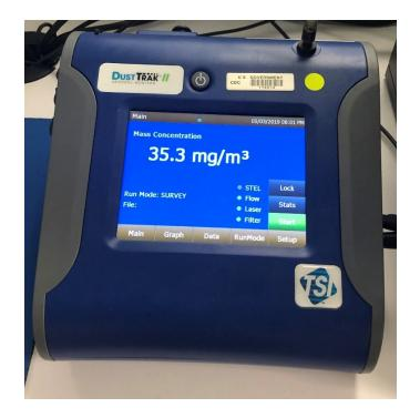
Figure 3: DustTrak II Aerosol Monitor
