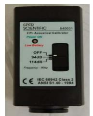
Figure 4. Acoustical calibrator (Sper Scientific model 840031)
