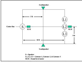
Figure 1. Modified Rhyme Test setup diagram
