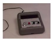
3.1.1. Electric time, calibrated to hundredths of a minute (Precision Scientific) or equivalent.
