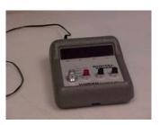
3.1.2. Electric timer, calibrated to hundredths of a minute (Precision Scientific Company) or equivalent.
