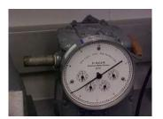
3.1.3. Singer Dry Test Meter (Model 806) one cubic foot per revolution or equivalent.
