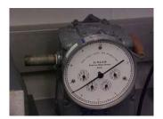
3.1.3. Singer Dry Test Meter (Model 806) one cubic foot per revolution of proper ranger or equivalent.
