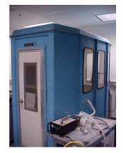
3.1.15. Corn Oil Generator and Chamber - Dynatech Frontier Enterprises Model 260 - (May be substituted for No. 3.1.8., above) or equivalent.
