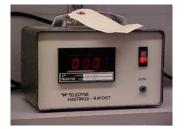
3.1.16. Teledyne Hastings - Ray Dist Mass Flow Meter - Model NAHL-25 (May be substituted for No. 3.1.13., above) or equivalent.
