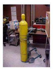
3.1.10. A 300 cubic foot gas cylinder of compressed air or equivalent.
