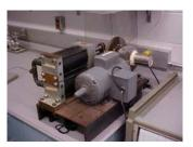
3.1.2. Mechanical Breather with 622 Kg.m/min. Cam as per U.S. BOM Drawings C-1748 (3/17/69) Breathing Machine and B-1198 (3/6/69) Breathing Cam or equivalent.
