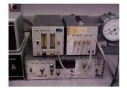
3.1.2. Applied Electrochemistry Oxygen Analyzer - Model S-3A or equivalent.
