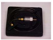
3.1.4. Bruel and Kjaer Accelerometer - Model 4384 or equivalent.
