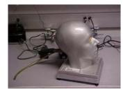
3.1.2. ISI Anthropometric Test heads with tube for measuring breathing resistance and air flows - Model SR-085 or equivalent.
