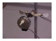
3.1.3. Temperature compensated pressure transducer (Validyne Engineering Model No. DP45) or equivalent.
