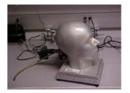
3.1.3. ISI anthropometric test head with tube for measuring breathing resistance (International Safety Instruments - Model SR-085) or equivalent.
