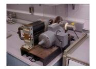
3.1.2. Mechanical Breather with 622 Kg.m/min. Cam as per U.S. BOM Drawings C-1748 (3/17/69) Breathing Machine and B-1198 (3/6/69) Breathing Cam or equivalent.
