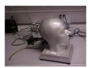
3.1.3. ISI anthropometric test head with tube for measuring breathing resistance (International Safety Instruments - Model SR-085) or equivalent.
