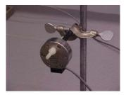
3.1.4. Temperature compensated pressure transducer (Validyne Engineering Model No. DP45) or equivalent.
