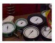
3.1.2. A Helicoid calibrated pressure gauge and connecting fittings or equivalent.
