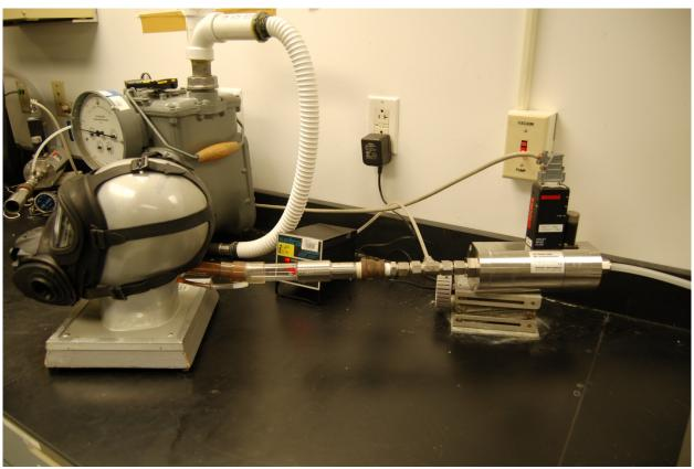
Figure 1: Exhalation resistance setup
