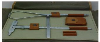
Figure 2, Facial Size Measurement Calipers
