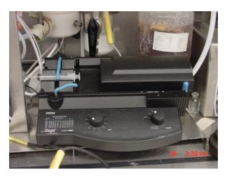
Picture 4: Syringe pump, Sage Model M365
