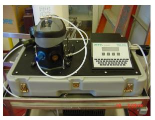
Picture 2: Leak detector Model TDA-99M
