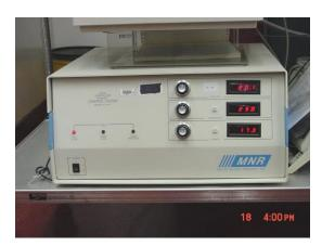
Picture 5: Flow-Temperature-Humidity Control System
