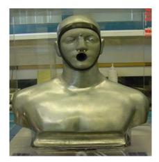
Picture 1. SiMulant Agent Resistant Test MANikin (SMARTMAN)
