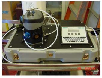
Picture 2: Respirator Leak Detector, Model TDA-99M
