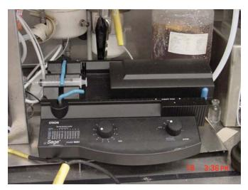
Picture 4: Syringe pump, Sage Model M365
