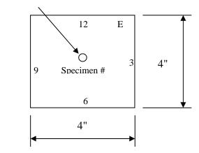
Figure 6. Four (4) reading positions/clock method.
