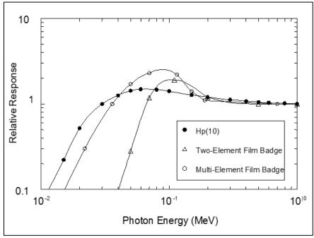
Figure 6-1. Comparison of Hp(10) for photons with energy responses for sensitive DuPont 502 emulsion in two-element film badge [Pardue et al. 1944] and sensitive DuPont 555 emulsion in multielement film badge [Thornton et al. 1961].
