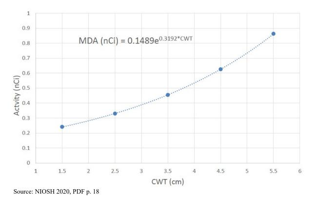
Figure 7-1: MDA for Pb-212 as a Function of Chest Wall Thickness (CWT)
