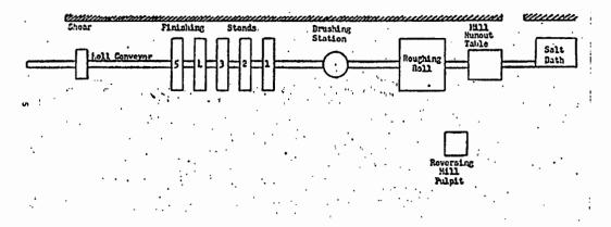
Figure 2. Superior Steel uranium mill layout (ORNL 1981).
