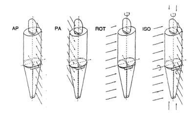
Figure 4.2 Exposure geometries of an anthropomorphic phantom extracted from ICRP 74 (1996)
