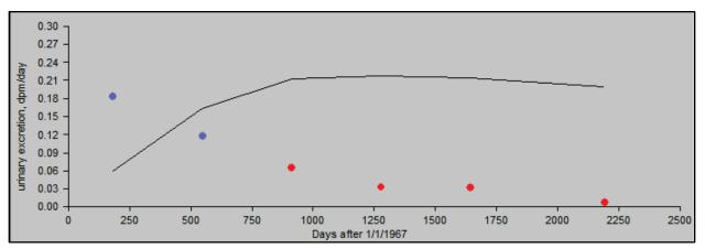
Figure A-9. Predicted plutonium gross alpha bioassay results calculated using IMBA-derived plutonium gross alpha intake rates (line) compared with measured bioassay results (dots), 50<sup>th</sup> percentile, 1967 to 1968, Type S.
