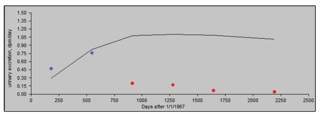
Figure A-12. Predicted plutonium gross alpha bioassay results calculated using IMBA-derived plutonium gross alpha intake rates (line) compared with measured bioassay results (dots), 84<sup>th</sup> percentile, 1967 to 1968, Type S.
