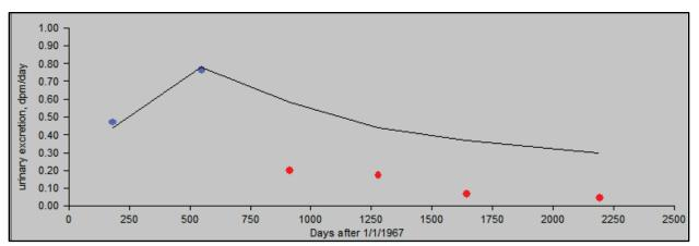
Figure A-4. Predicted plutonium gross alpha bioassay results calculated using IMBA-derived plutonium gross alpha intake rates (line) compared with measured bioassay results (dots), 84<sup>th</sup> percentile, 1967 to 1968, Type M
