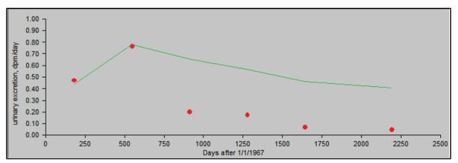
Figure A-8. Predicted plutonium gross alpha bioassay results calculated using IMBA-derived plutonium gross alpha intake rates (line) compared with measured bioassay results (dots), 84<sup>th</sup> percentile, all years, Type M
