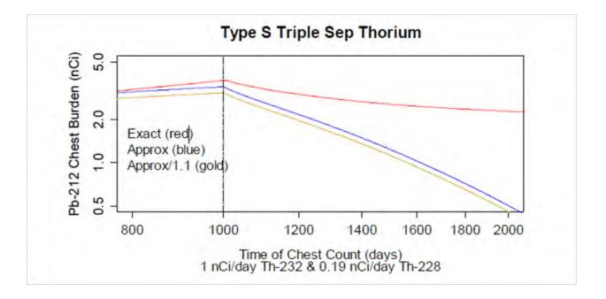
Figure 10. Pb-212 chest burden during and following a 5000-day chronic inhalation intake of Type S thorium having a Th-228 to Th-232 ratio of 0.19 : 1. The vertical dashed line is at t = 5000 days.
