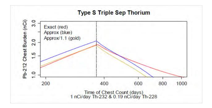
Figure 9. Pb-212 chest burden during and following a 1000-day chronic inhalation intake of Type S thorium having a Th-228 to Th-232 ratio of 0.19 : 1. The vertical dashed line is at t = 1000 days.
