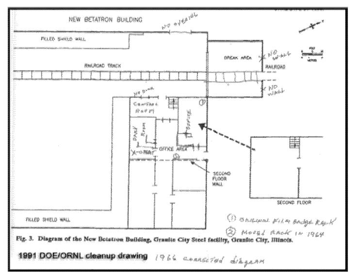
LEGEND. New Betatron building drawing by ORNL/ DOE 1991 during the GSI cleanup. Map has been annotated in red to show the true situation that existed 1964-1966 with GSI Radiographer film badges stored in locations (1) and (2)away from the Betatron operating console area marked "control room" on this diagram. Source JTD 3/12.
