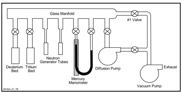
Figure 2-7. Neutron tube tritium loading manifold.
