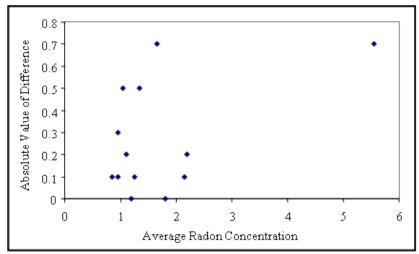
Figure 5-1. Absolute differences between duplicate radon measurements [47].
