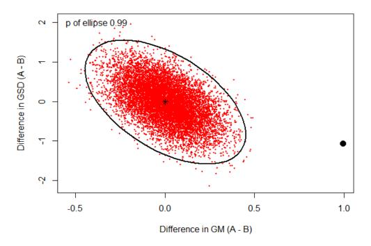
Figure A-9. Monte Carlo permutation test of coworker models for Stratum A and Stratum B (work area) using a bivariate normal probability ellipse. The large dot in the lower right corner corresponds to the observed differences in GM and GSD. The strata are significantly different at the  $\alpha$  = 0.05 confidence level.
