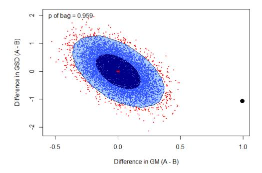
Figure A-10. Monte Carlo permutation test of coworker models for Stratum A and Stratum B (work area) using nonparametric bagplot probability polygon. The outer polygon encloses ~95% of the points whereas the inner polygon encloses ~50% of the points. The strata are significantly different at the  $\alpha$  = 0.05 confidence level. The large dot in the lower right corner corresponds to the observed differences in GM and GSD.
