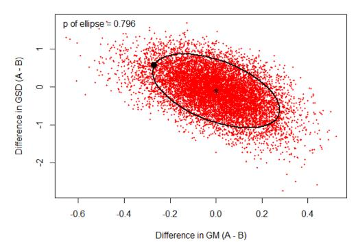
Figure A-4. Monte Carlo permutation test of coworker models for Stratum A and Stratum B (job title) using a bivariate normal probability ellipse. The large dot on the ellipse corresponds to the observed differences in GM and GSD. The p-value of the test is 1 - 0.796 = 0.204, which means the strata are not significantly different at the  $\alpha$  = 0.05 confidence level.
