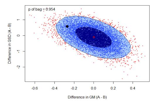
Figure A-5. Monte Carlo permutation test of coworker models for Stratum A and Stratum B (job title) using a nonparametric bagplot probability polygon. The outer polygon encloses ~95% of the points and the inner polygon encloses ~50% of the points. The strata are not significantly different at the  $\alpha$  = 0.05 confidence level. The large dot inside the outer polygon corresponds to the observed differences in GM and GSD.
