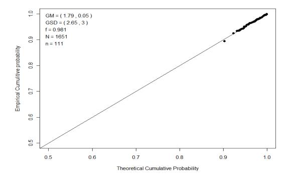
Figure A-16. P-P plot where the points are the uncensored data. The GM and GSD each have two values, one for each distribution in the mixture. For example, the first distribution has a GM = 1.79 and a GSD = 2.65. If the model fits the data, the data should fall on a straight line through the origin with a slope of 1.
