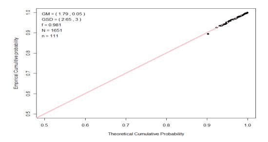
Figure A-17. P-P plot where the dark points are the uncensored data and the smaller light points are the imputed values for the censored data. The GM and GSD each have two values, one for each distribution in the mixture.
